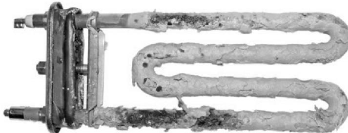
Hard water causes a build-up of limescale on heating elements, as in the picture on the left.
