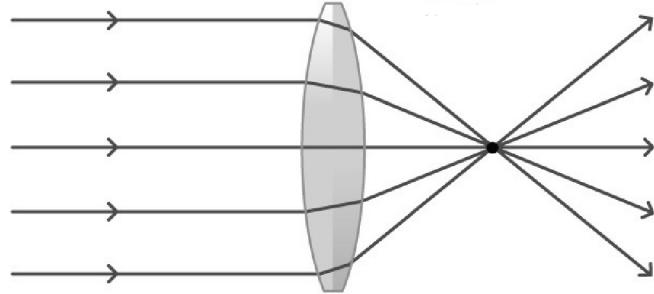
The picture shows a converging lens with rays of light passing through it.
